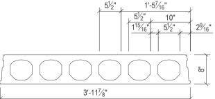
1- Dead Load, 87 psf grouted weight of structural unit.
