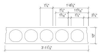
1- Dead Load, 97 psf grouted weight of structural unit.
